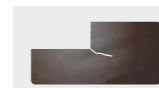
Cutting a laminate sheet at an angle of 90 degree leads to development of cracks in corner after pasting. Therefore it is advisable to avoid cutting at an angle of 90 degrees.
